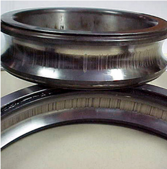
Typical bearing fluting caused by EDM
